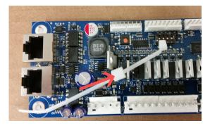
3. Route the cable tie around and through D9 and then loop it back to the other end.
