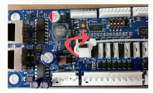
4. Secure the cable tie by hand (no tools) snug enough to capture the spacer between the D9 and Q4 tabs.
