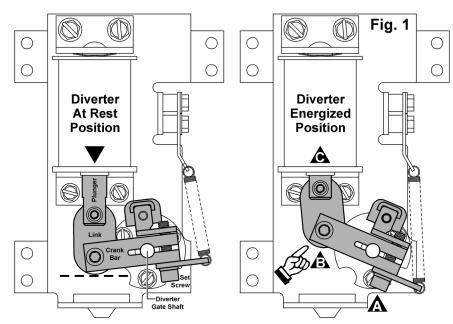
**Step 1:** Under the Playfield, using a 5/32" Allen Wrench, loosen the Set-Screw on the Crank Bar *just enough so that the Diverter Paddle can move with a gentle amount of force. Ref. Fig. 1-A.*
