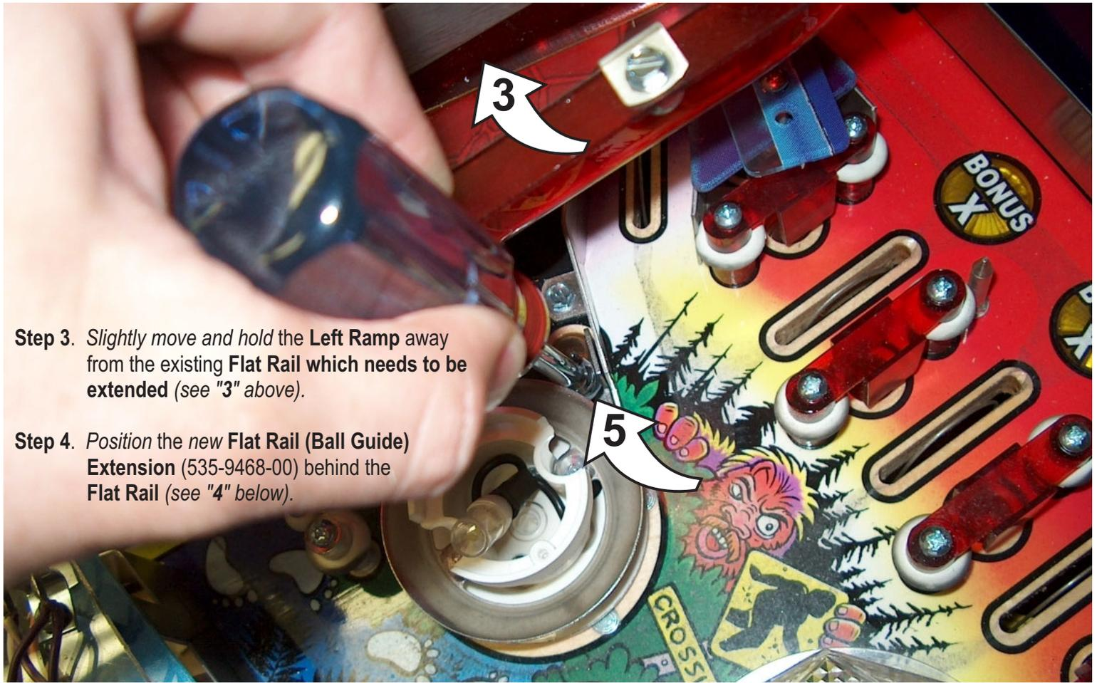
**Step 3.** Slightly move and hold the **Left Ramp** away from the existing **Flat Rail** which needs to be **extended** (see "3" above).
