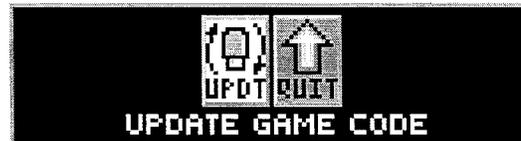
TO UPDATE GAME CODE, MOVE DIP SWITCH #8 TO 'ON' (on CPU/SND PCB). PERFORM CPU / SND PCB RESET PRESS THE **WHITE BUTTON**. FOLLOW ON-SCREEN PROMPTS (REVIEW INSIDE COVER).
