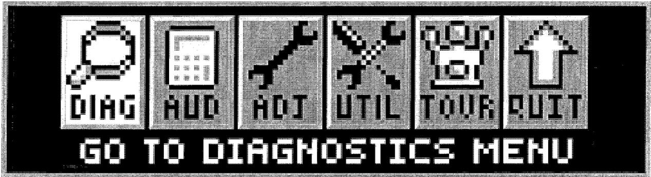
To initiate, from the **MAIN MENU**, select the "DIAG" *Icon*. The **DIAGNOSTICS MENU** provides tests for switches, coils, flash lamps, lamps, sounds and dots in the Dot Matrix Display. Each feature may be tested manually or automatically after entering the **SERVICE MENU** (see *Service Menu Introduction Section*).
