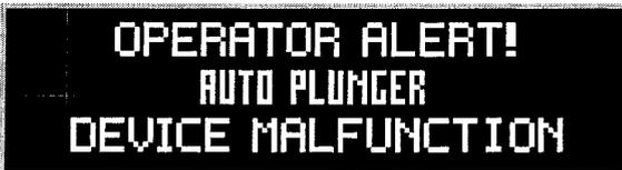
This **alert display** is shown momentarily during **Game Mode** or **Power-Up** to alert the operator of a device malfunction (device or mechanism doesn't energize or is energized repeatedly).
