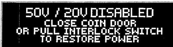
This **audible / visual alert display** is shown when the **50V / 20V Power** is disabled (by opening the **Coin Door**). **PULL OUT THE INTERLOCK SWITCH ONLY WHILE IN THE SERVICE MENU FOR COIL OR SWITCH TESTING & BURN-IN WHEN THE COIN DOOR IS REQUIRED TO STAY OPEN FOR SERVICE BUTTON USE!** Pulling out the Power Interlock Switch or
