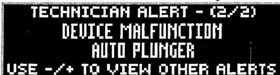
**NOTE ON DEVICE MALFUNCTION :** While in **TECHNICIAN ALERTS MENU**, if the following is displayed, the game has detected a "device malfunction." Check the device indicated (*coil and/or switch*).
