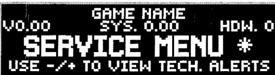
Upon entering the **SERVICE MENU**, if an asterisk " \* " is displayed after the words "SERVICE MENU," the game has detected possible faulty devices, switches and/or missing pinballs. Press the either of the **Red Buttons** (short-cut to the **TECHNICIAN ALERTS MENU**) or continue into the **SERVICE MENU** (press the **Black Button** again), select the "DIAG" *Icon*
