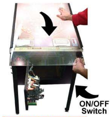
13. Open the Coin Door and pull the YELLOW HANDLE to the LEFT and at the same time pull up on the FRONT TOP MOLDING and remove. The GLASS can now be pulled out towards you and removed. TAKE CARE while moving; set glass on a safe surface.
