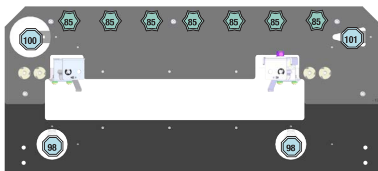
Figure 3.3.5. Playfield back panel lighting locations.
