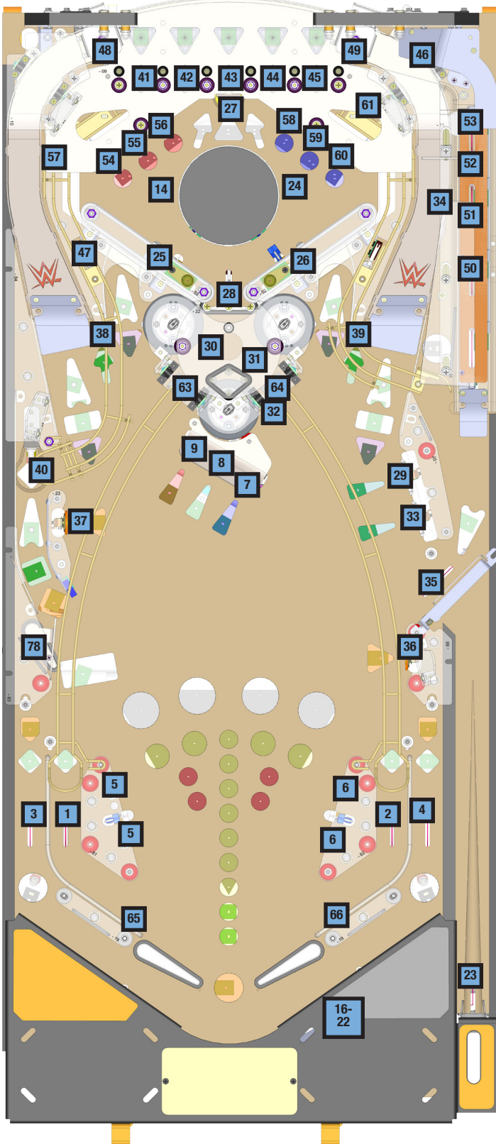
Figure 3.4.1. Switch locations, playfield top view
