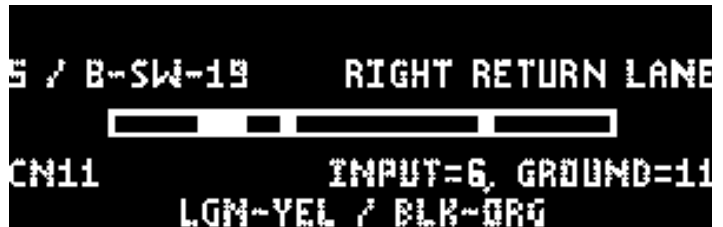
Switch Test screen (Small squares indicate closed switches.) When you open the test, closed ball trough switches are normal.
