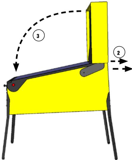
2. Remove the backbox securing bolts
