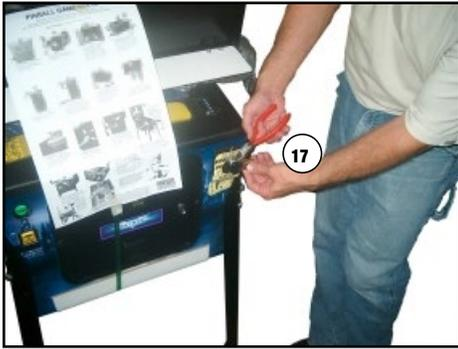
15. Cut nylon strapping and remove protective strap corner guards.
