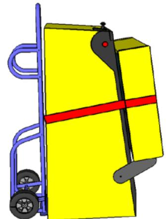
10. Secure all loose parts and transport with a hand truck in the upright position.
