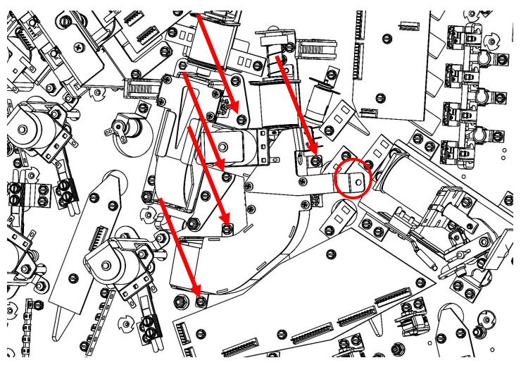
5.3. Plug in the opto connectors, post connectors, and switch connectors for the side scoop. See image below for connector locations.
