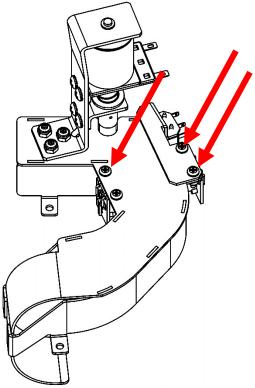
4.2. Using the #2 phillips screwdriver, install the new switch assembly (Item 3) as shown below.
