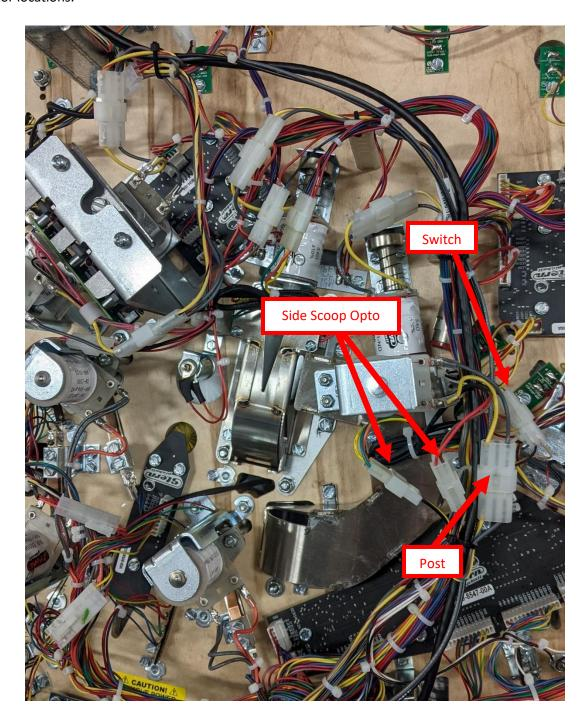
3.4. Using a 1/4" nut driver, remove the 5X wood screws for the side scoop. Set aside the wood screws, and side scoop for use in section 5.2.
