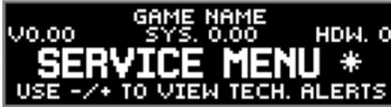
After selecting this icon, the display will indicate the alert(s). If there are 2 alerts present, the display will indicate (1/2) with the 1st alert on display. Press the red [+>] button to view the second alert (2/2). The second number in the parenthesis after the slash indicates how many alerts total are present. To return to the diagnostics menu, press the green [BACK] button.
