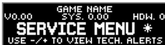
Upon entering the service menu, if an asterisk “\*” is displayed after the words “SERVICE MENU”, the game had detected possible faulty devices, switches, and/or missing pinballs. Press either of the red buttons (short-cut to the technician alerts menu) or continue into the service menu (press the black button again), select the “DIAG” icon and “TECH” icon for the technician alerts information.
