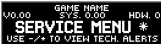
Upon entering the service menu, if an asterisk "\*" is displayed after the words "SERVICE MENU", the game has detected possible faulty devices, switched, and/or missing pinballs. Press either of the red buttons (short-cut to the technical alerts menu) or continue into the service menu (press the black button again), select the "DIAG" icon and "TECH" icon or the technical alerts information.
