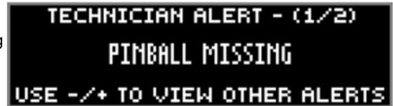
During gameplay a pinball can get trapped or stuck. If after approximately 15 seconds of inactivity or “no scoring”, Ball Search is started. Note: If the pinball is in the plunger lane or “held” on the flipper, no ball search will be performed. The game will perform one ball search in an attempt to “find” or free-up the pinball.
