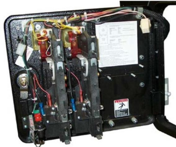
The four buttons (inside the coin door) have dual functions depending on if you have entered the Service Menu or not.
