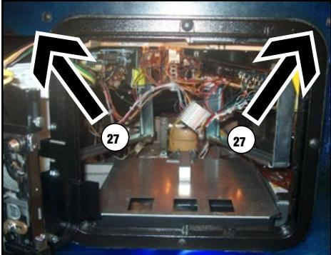
27. Reach inside the cabinet and lift the two latches located on either side of the coin door.
