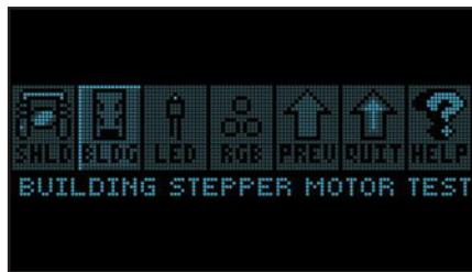
2. The BUILDING STEPPER MOTOR TEST has two modes, MOVE and ADJUST. The test menu can be toggled between these two modes by pressing START on the game cabinet.
