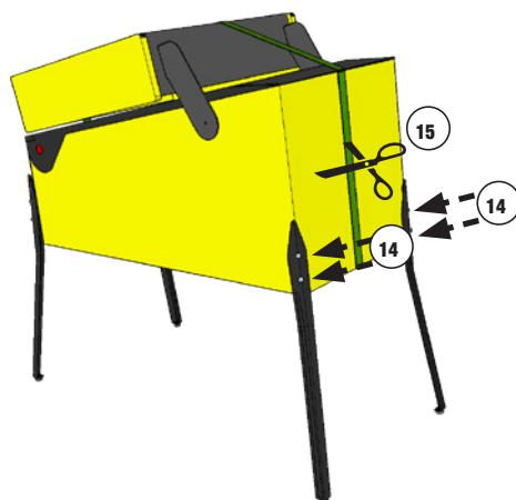
8. Install front legs using the bolts removed from the cabinet. Secure tightly.
