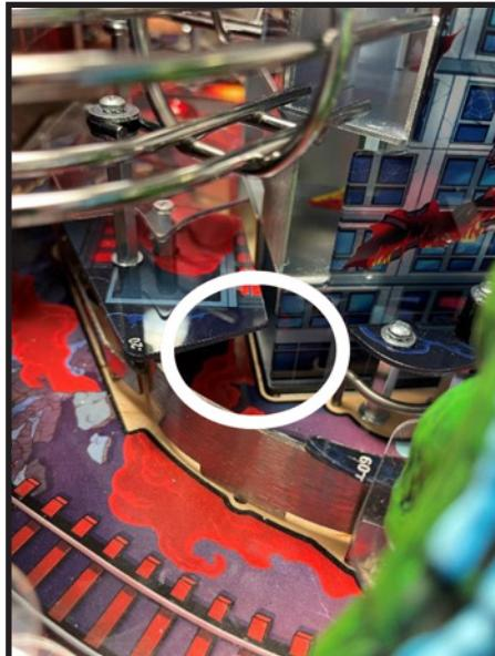
2. Using a 11/32" nut driver, manually turn the two 8-32 nuts indicated below until the front edge of Floor 1 is level with the playfield.
