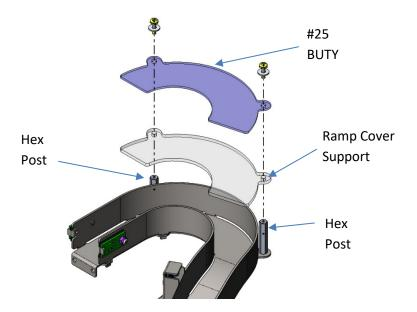
4.2. Re-tighten the hex posts with a ¼" nut driver. Install thick clear RAMP COVER SUPPORT item 3 and arted BUTY #25 on top of the RAMP COVER SUPPORT. Secure the assembly with two #6 flat washers and two #6-32 x ½" Phillips Pan Head screws provided in kit. Tighten securely.
